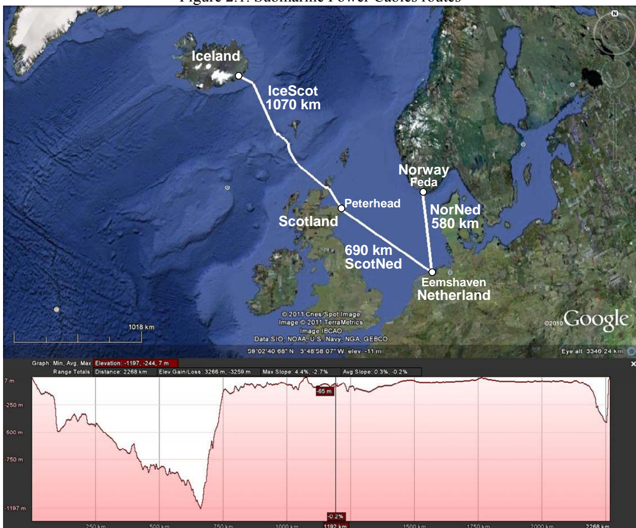
Figure 2.1. Submarine Power Cables routes
